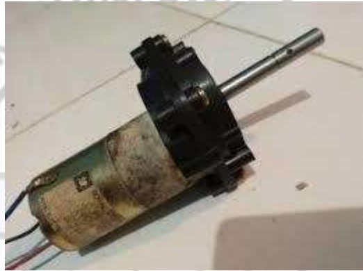
Gambar 2.9 Motor DC Gearbox KR13091
