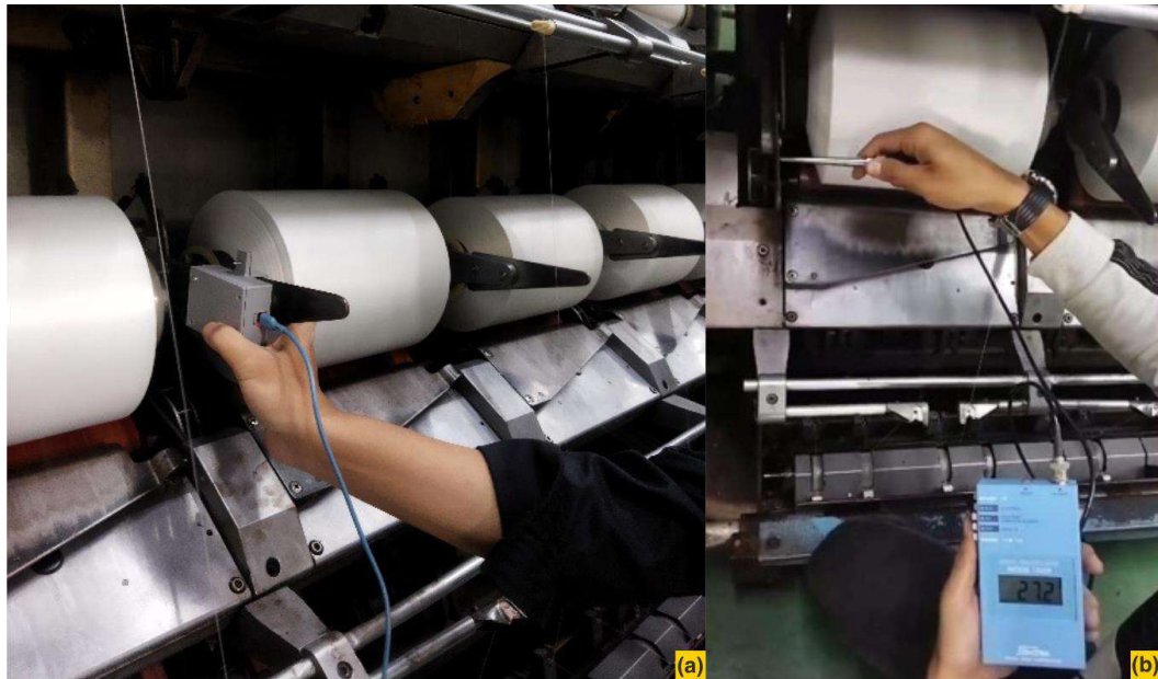
Figure 2. The process of installing (a) and calibrating (b) the sensor on the DTY machine spindle
