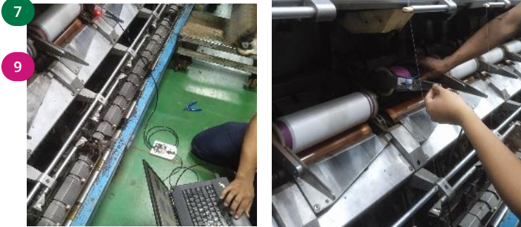
Fig. 9. Sensor mounting position on spindle arm.
