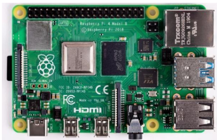
Fig. 2. Raspberry Pi 4 as the main controller
